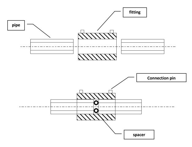
Electrofusion welding process shall be carried accordingly to below general instructions and specific recommendations provided by the fitting manufacturer:
